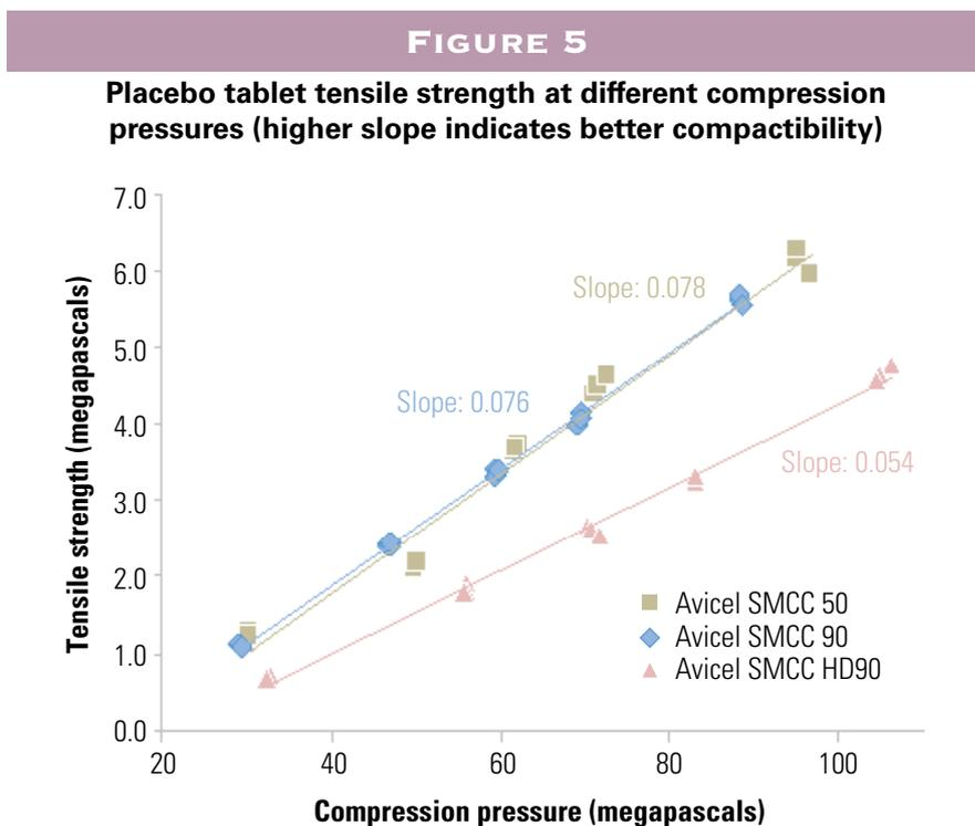
suitable for DC tableting and continuous manufacturing processes than traditional MCC.
