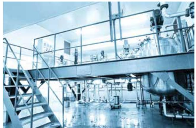
**Photo 1:** Ensure that the room in which new equipment is to be installed has the proper drain system with floor connections next to the intended equipment location or be prepared to spend big dollars and allow for significant downtime to trench new drains.
