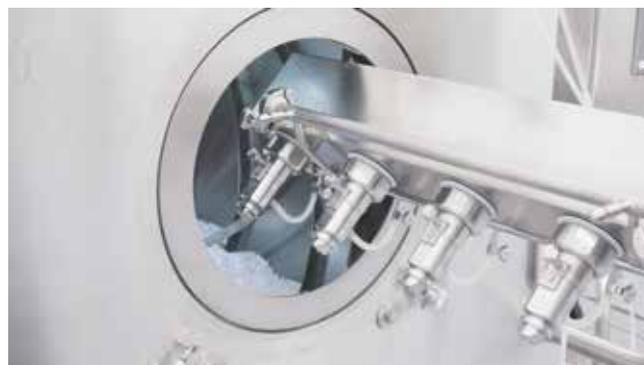
**Photo 1:** Manufacturing monolithic-matrix tablets uses simple equipment and is relatively quick and inexpensive. Delayed release can be achieved by applying a coating that prevents the tablets from immediately dissolving in the stomach.
