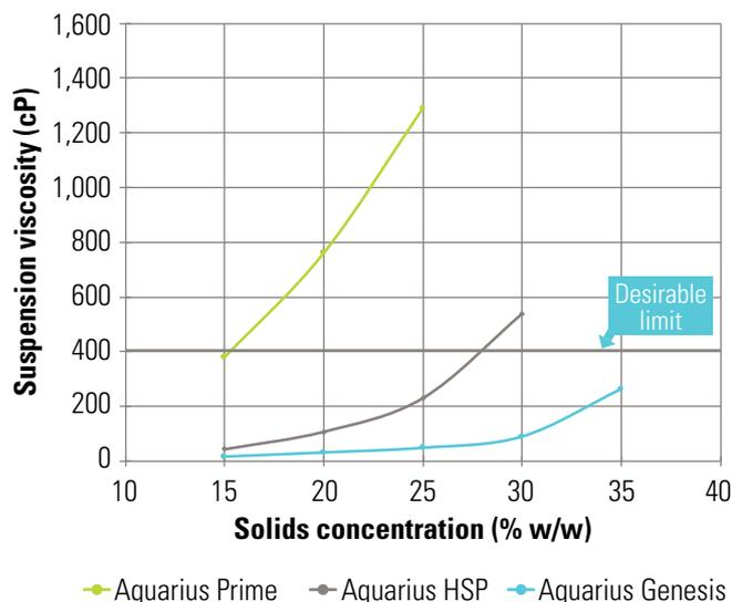
(sprayed at 12.5 percent w/w solids) to that of an intermediately high-solids film coating formulation (Aquarius Preferred HSP, sprayed at 20 percent w/w solids) and an ultra-high-solids film coating formulation (Aquarius Genesis, sprayed at 35 percent w/w solids).
