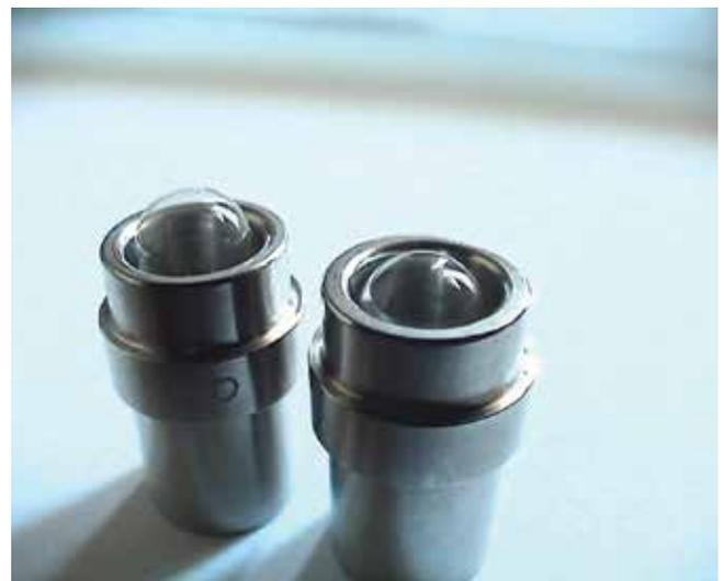
**Photo 1:** This photo shows caps from two different capsule suppliers seated in tooling (IMA Zanasi 40). Note the difference in cap length. Switching between these two capsules would require adjustment to the counter bearing to prevent cap tucks.
