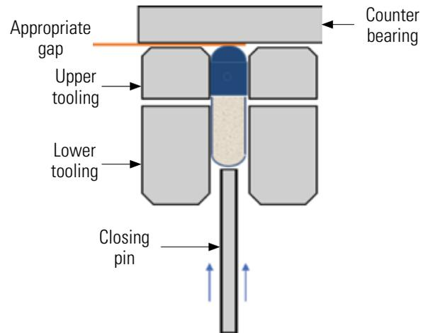
top of the cap dome. An excessive gap allows the cap to travel up and out of the stabilizing walls of the tooling, which can cause the cap to rock from side to side and collide with the capsule body during closing, as shown in Figure 1a. A small gap allows the cap to move very slightly, for self-centering as the body enters the cap, but keeps the cap from rocking laterally (Figure 1b).
