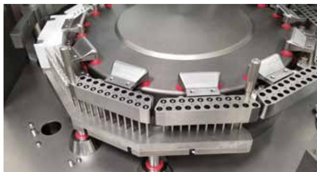
**Photo 3:** Be sure to check the alignment of the turret in relation to the closing station during machine setup to prevent damaged capsules. (Unit pictured is a Bosch 3005.)
