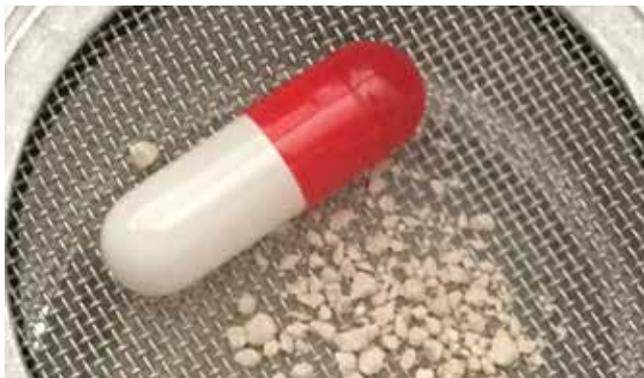
**Photo 2:** Coarse granules in the fill material can distort the capsule body, preventing smooth closing and causing cap tucks.
