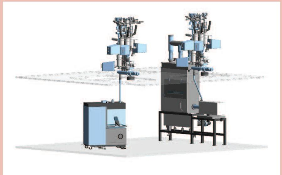
Patheon's continuous manufacturing line will use modular components to perform dry granulation, wet granulation, tableting, and capsule filling. This rendering shows the direct-compression and wet granulation modules positioned below a manifold of six feeders.
