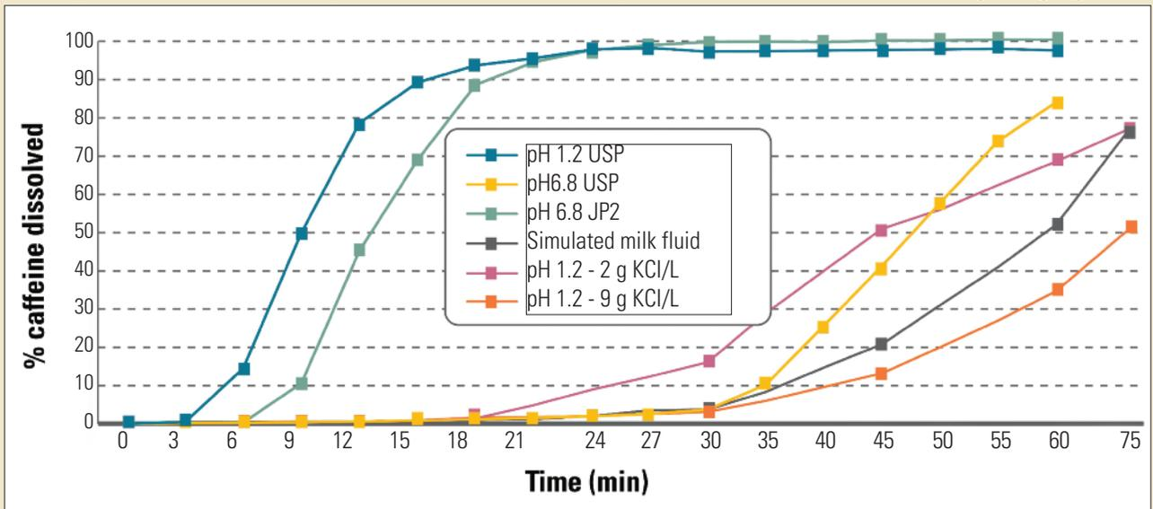
a. In vitro dissolution of caffeine filled into HPMC capsules made with gelling agents (kappa-carrageenan and potassium chloride).
